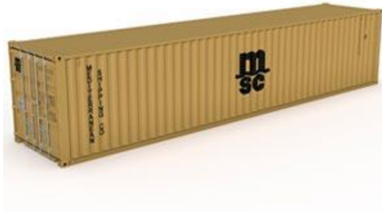
PICTURE 2. A 40' standard freight container (MSC 2017a)
