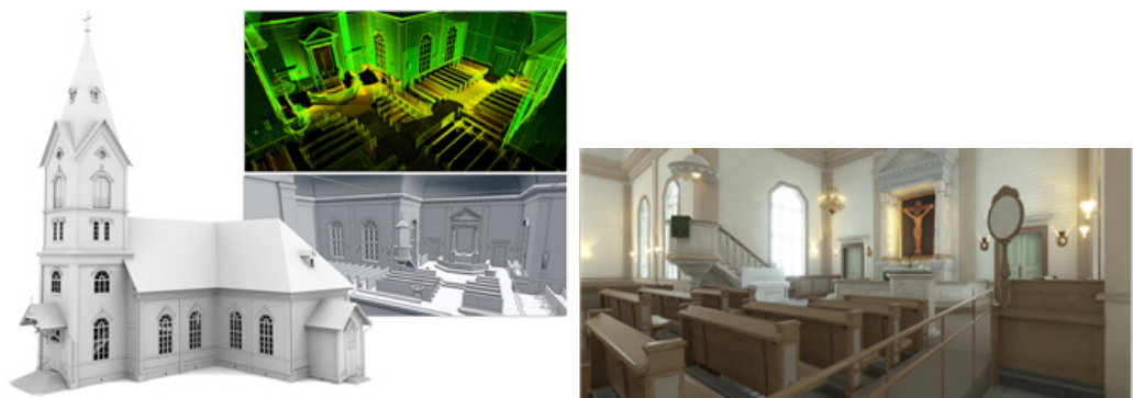
FIGURE 5. Ylivieska church as a point cloud, 3D model and virtual model for VR and mobile devices
