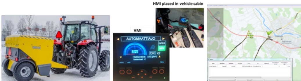
FIGURE 23. Location Aware towable gritter with GPS tracking and cloud services
