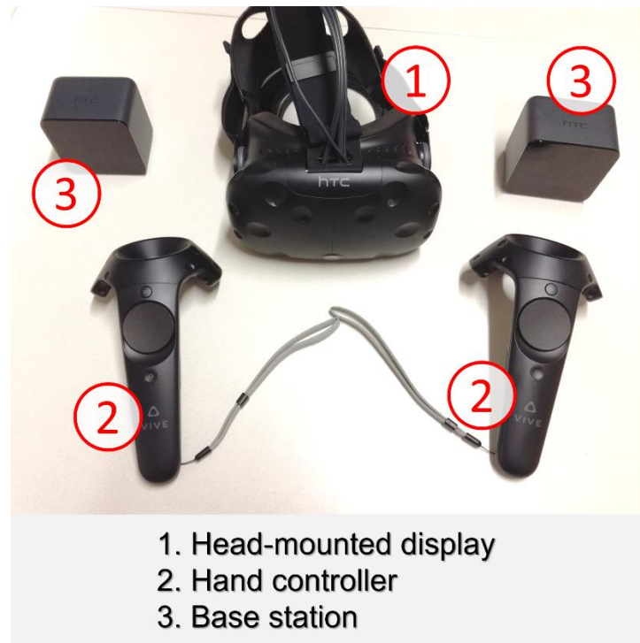
Image 2. HTC Vive's main components.
