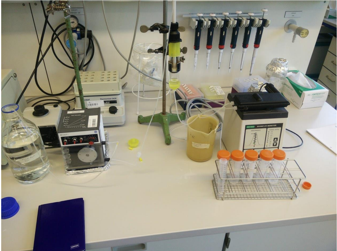
Figure 14. Setup for Cycle 0 IMAC being washed with Milli-Q water.
