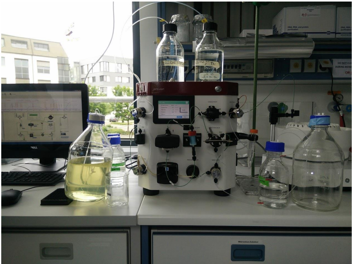
Figure 15. setup for IMAC with Äkta start in loading phase.
