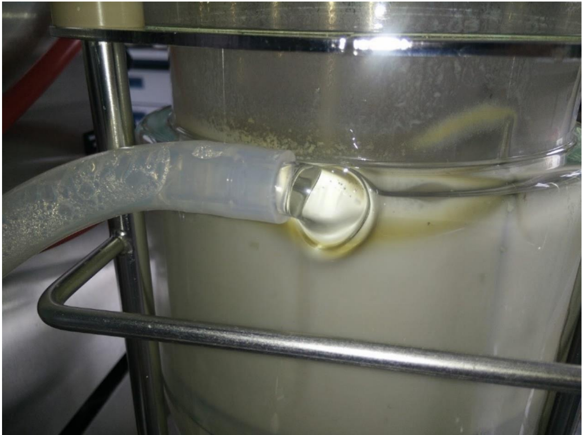
Figure 34. Reactor contamination seen as a yellow culture adhering to the reactor wall and baffle.
