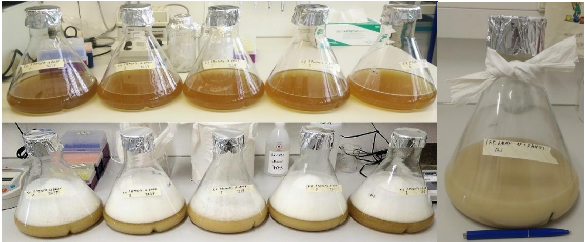
Figure 10. flasks before (top left) and after (bottom left) glycerol growth phase without AF; flask with AF in methanol induction phase (right).
