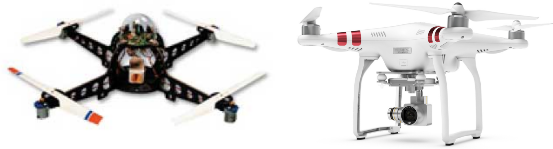
Figure 2.2: Left: the original Draganflyer, one of the first commercial quadrotors [Draganfly Innovations, 2016]. Right: the DJI Phantom 3, currently one of the most ubiquitous quadrotors [DJI Technology, 2017].
