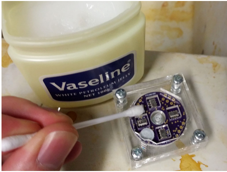
1. Assemble laser cut mould and apply release agent
