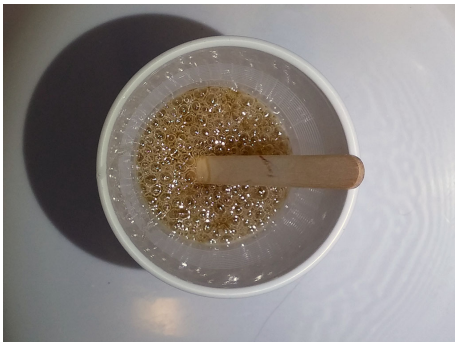
3. De-gas in a vacuum chamber until bubbles stop
