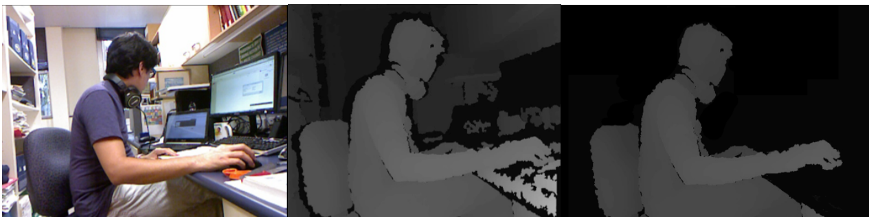
Figure 1. Three stages of image processing for depth information. Raw photo (Left), heat map based on depth camera values (brighter is closer, darker is farther away) (Middle), and segmented image where only the pixels at a pre-determined distance are presented (Right). Images are taken using the Microsoft Kinect sensor.
