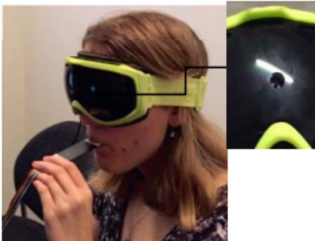
Figure 1. Blackened out ski goggles were used to house the input camera (Left). A modified webcam was fitted into the back of goggle lens (Right). The ski goggles provided a comfortable and stable base to ensure the camera position remained consistent throughout the tasks.
