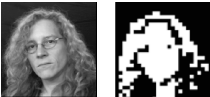
Figure 4. Image processing sequence. Initial camera image is converted to grayscale (Left), downsampled to 32x32 pixels, then the individual pixel values are thresholded to determine which pixels will be active or turned off (Right). The threshold value can be adapted as necessary depending on the amount of light present in the environment. E.g. in outdoor daylight settings the overall threshold may need to be lowered so that the contrasts within the object are more clear.
