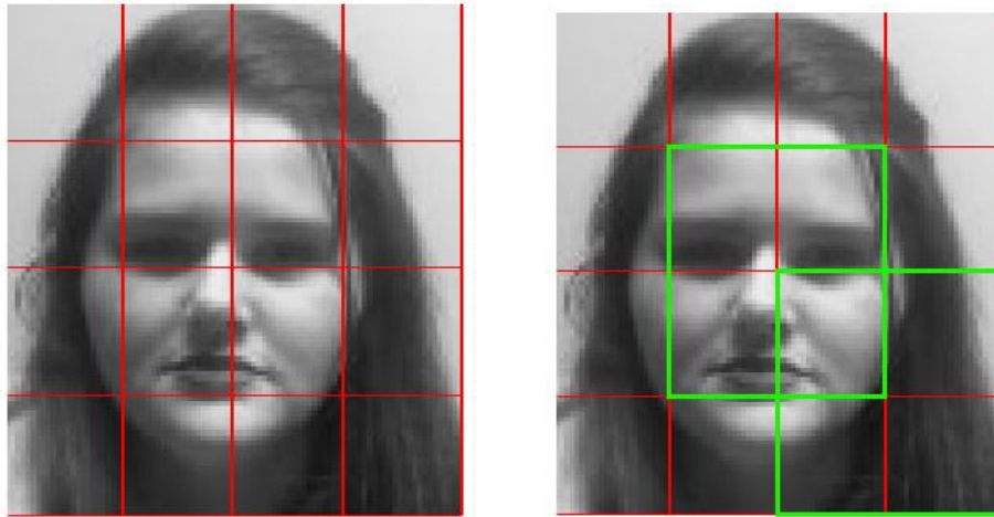
(a) An image divided into cells of size 8 \times 8 . (b) Cells grouped into blocks with 50% block overlapping rate.
