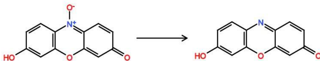
Figure 2.9: Photocatalytic ink resazurin reduction to resorufin (blue to pink colour change).
