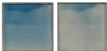
Figure 6.16: Annealed \text{Ti}_{0.99}\text{Ga}_{0.01}\text{O}_2 film before and after six hours irradiation.
