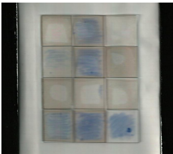
Figure 4.28: Basic blue 66 ink degradation subsequent to three hours UV irradiation on; a) nominally undoped \text{TiO}_2 , b) \text{Ti}_{1-x}\text{O}_2:\text{Ag}_x (99:1), c) \text{Ti}_{1-x}\text{O}_2:\text{Ag}_x (19:1), d) \text{Ti}_{1-x}\text{O}_2:\text{Al}_x (99:1), e) \text{Ti}_{1-x}\text{O}_2:\text{Al}_x (19:1), f) \text{Ti}_{1-x}\text{O}_2:\text{Hf}_x (99:1), g) \text{Ti}_{1-x}\text{O}_2:\text{Hf}_x (19:1), h) \text{Ti}_{1-x}\text{O}_2:\text{Sn}_x (99:1), i) \text{Ti}_{1-x}\text{O}_2:\text{Sn}_x (19:1), j) \text{Ti}_{1-x}\text{O}_2:\text{V}_x (99:1), k) \text{Ti}_{1-x}\text{O}_2:\text{V}_x (19:1) and l) a blank quartz substrate.
