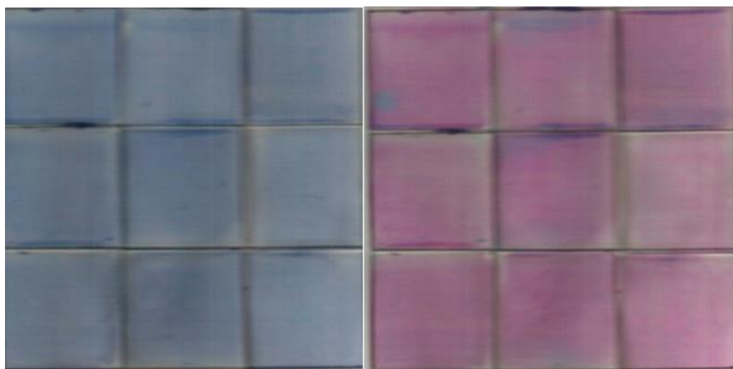
Figure 5.2: Resazurin ink degradation (before and after UV light irradiation) on Ti_{1-x}O_2:Sn_x (19:1).
