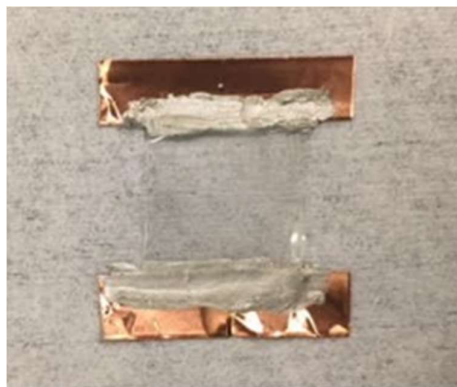
Figure 5.7 Photograph of a crossed silver/zinc oxide nanowire structure.
