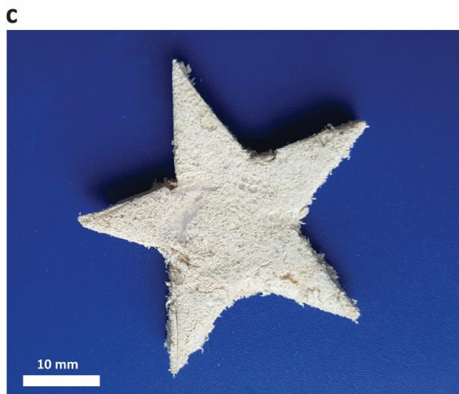
332 Figure 5. a) Stress-strain curves during uniaxial compression upon first compression; each 333 curve corresponds to a different sample. b) Thermal and mechanical properties. c) 334 Demonstration of the ability to shape the pullulan-silica aerogel composites by cutting.
