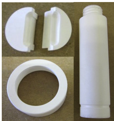
Fig. 4. Modular boron nitride crucible used in this work (courtesy Edmund Bühler, Germany).
