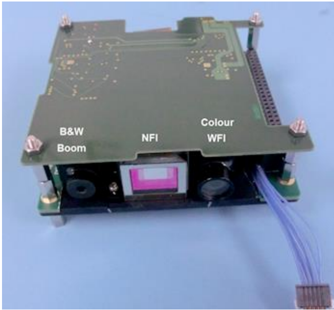
Figure 10: Assembled FM of C3D2 (left) and integrated onto the 3U CubeSat Ain the lab (right)
