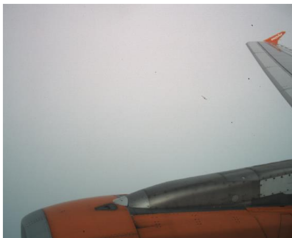
Figure 13: Image taken using a spare EM unit with the WFI during a “test flight” on an airplane above clouds to verify operation of the automatic exposure for an illumination level similar to that in-orbit
