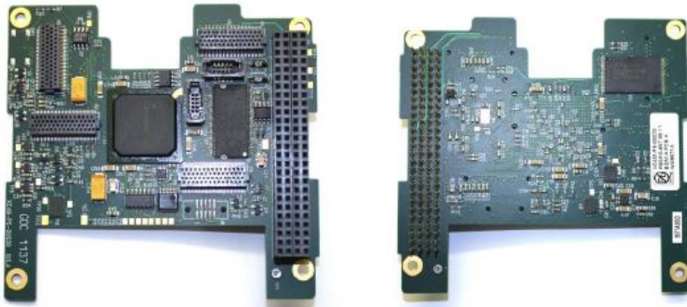
Figure 6: Photographs of the payload control electronics which were developed by XCAM
