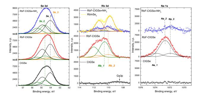
*Figure 3. Detailed XP spectra of the Rb 3d, Se 3d, and Na 1s of the CIGSe absorbers before the RbF-PDT, after the RbF-PDT, and after the NH3 etching of RbF-CIGSe.*
