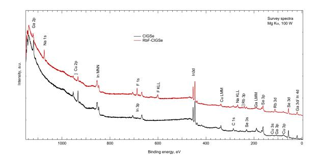
Figure 1. XP survey spectra of two vacuum transferred CIGSe absorbers prepared under the same conditions: before the RbF-PDT and after the RbF-PDT.
