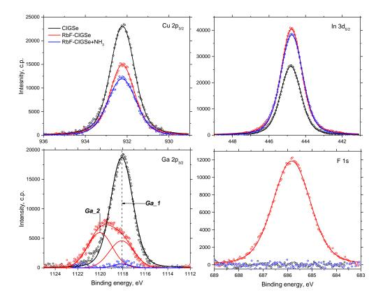
*Figure 2. Detailed XP spectra of the Cu 2p<sub>3/2</sub>, In 3d<sub>5/2</sub>, Ga 2p<sub>3/2</sub>, and F 1s of the CIGSe absorbers before the RbF-PDT, after the RbF-PDT, and after the NH<sub>3</sub> etching of RbF-CIGSe.*
