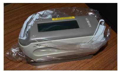
Figure 4.2. Contact spectrophotometer (CM-2600D, Konica Minolta, Japan) used for measuring dermatological patients. For biological protection it was repacked with a new plastic protector for every new patient. The transparent plastic covered the measure sensor ate the bottom of the instrument and therefore its calibration had to be made having g the plastic in account.
