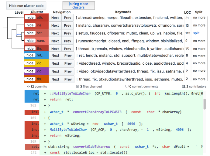
Figure 5: Features in fork DomAmato/ofxVideoRecorder ; tree view displaying hierarchical relation between split features; colors related code to features.
