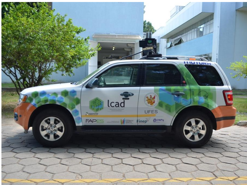
Figure 1: Intelligent Autonomous Robotic Automobile (IARA). A video of IARA's autonomous operation is available at https://goo.gl/RT1EBt . A description about the project is available at http://www.lcad.inf.ufes.br/wiki/index.php/IARA .
