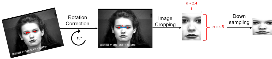
Figure 11: Spatial Normalization. The spatial normalization procedure comprises three steps: rotation correction, image cropping and down-sampling, in this order.
