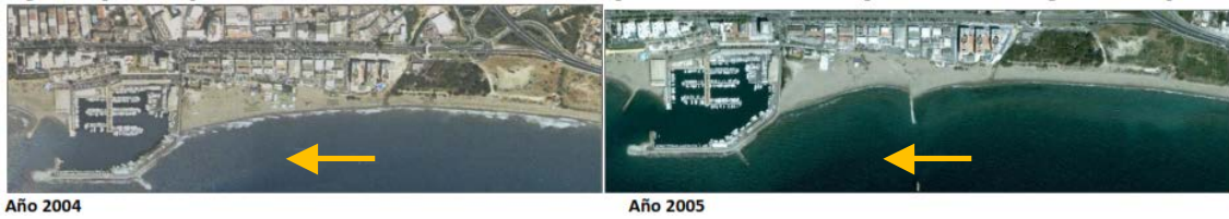
Fig. 11 El Cable Beach (Marbella, Spain). Direction of the clear ST, and variation of the shore alignment due to changes or works that concern the ST.
