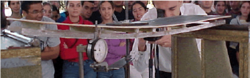
Fig. 2. Example of practical representation of the deformed shape of a beam due to a load
