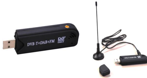
Fig. 3 RTL-SDR device used in the classroom and a simple antenna (comes with the SDR)
