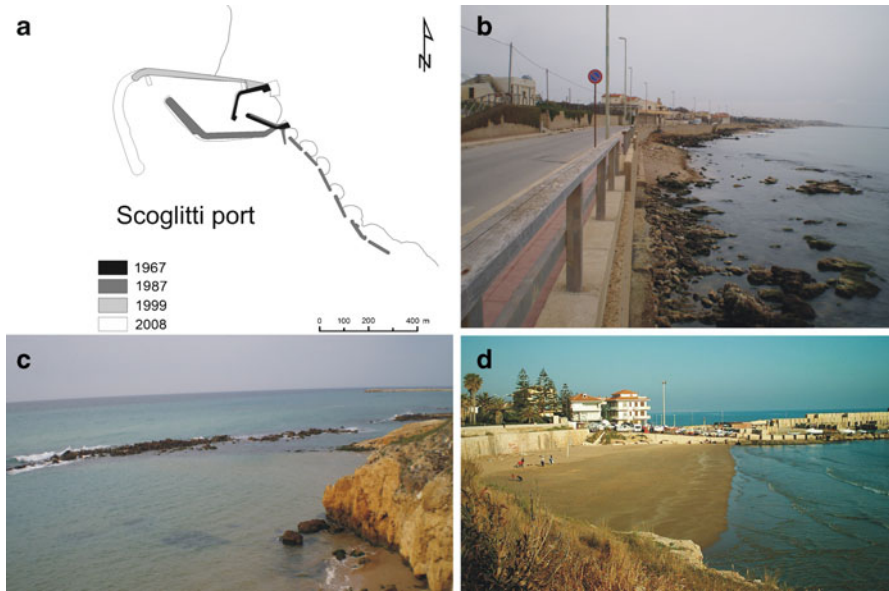
Fig. 13.3 Phases of Scoglitti port enlargement (a); littoral sector between P. Zafaglione and Scoglitti port, view from north to south (b, December 2010); southern breakwaters emplaced down-drift (south) of Scoglitti port (c, December 2010) and beach accretion up-drift (west) of the dock and haulage zone at Marina di Ragusa (d, April 2006)
