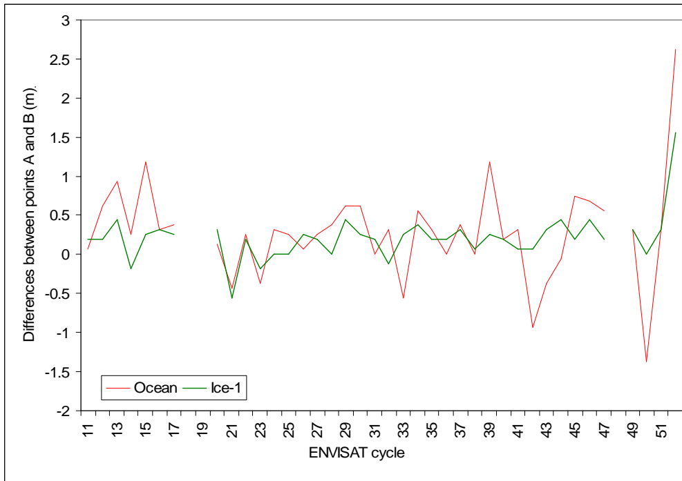
Figure 5.3. Time series comparison of corrected range differences between points A and B using Ocean (red line) and Ice-1 (green line) retrackerers. Units are in m.
