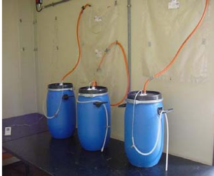
FIG. III.2. a) Reactores SEBAC
