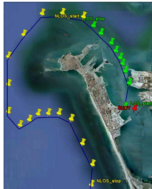
Figure 3. Fixed location of the transmitter buoy (red) and route followed by the receiver ship (blue) in the measurement campaign. Measurements carried out over green and yellow waypoints are considered LOS and NLOS, respectively.
