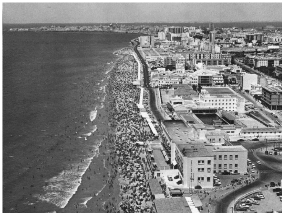
Fig. 3 Littoral coastline at the 80's . No berm or dry beach existed at high tide
