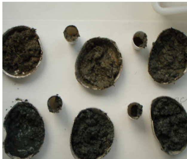
Fig 10: Separation of roots biomass from each core slice.
