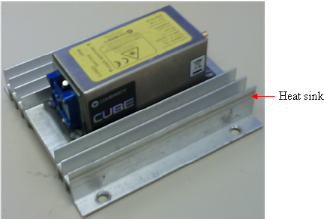
Figure 4.3: Photograph of a laser used to scan PV modules.
