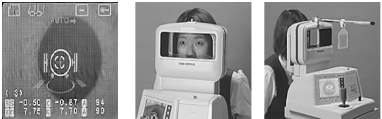
Figure 3.9. Instrument's LCD monitor display of pupil alignment (left), Binocular open view refraction at distance (middle), refraction at near (right). The Figure is reproduced from the operation manual for the Shin Nippon NVISION-K 5001 infrared open view refractometer.
