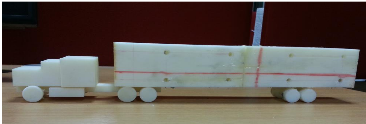
Figure 3-4: Wind-tunnel model of tractor semitrailer (scaled- ADAMS model)
