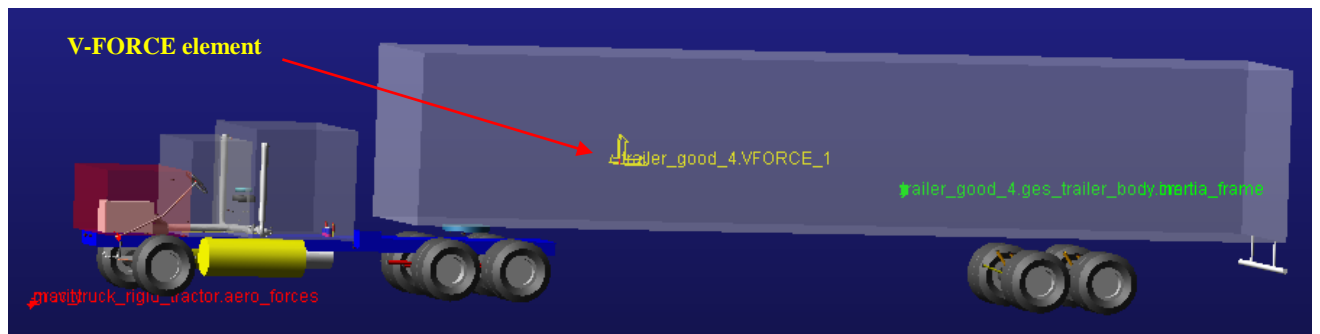
Figure 6-1: Aerodynamic center on ADAMS model
