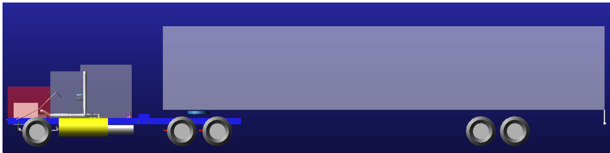
Figure 3-3 : Tractor semitrailer model built in ADAMS/Car
