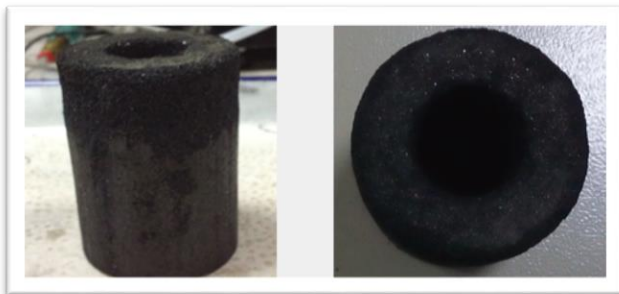
Figure 1 Molded coal with part hollow center for water invasion test; the hollow center is designed to hold the water container for the imbibition tests.
