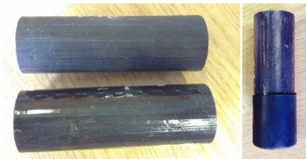
Fig.2. Preparation of the corroding samples: original iron bar, bar coated with PCB lacquer, coated bar with set heat shrink tubing
