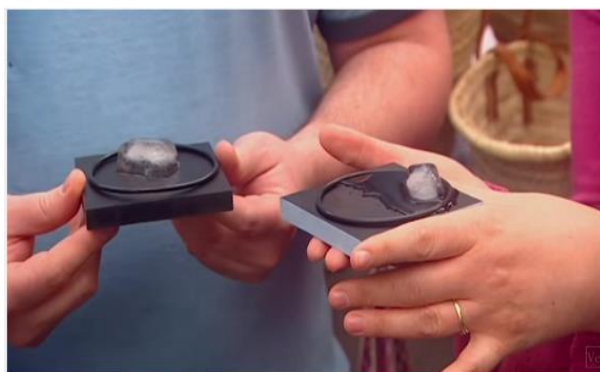
Figure 4-13: Heat conduction in different materials
