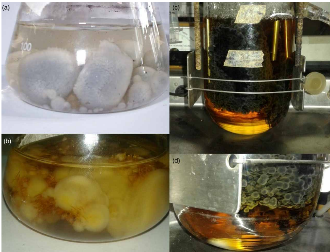
Figure 2 | Fungal growth: (a) no-carrier control after 15 days at laboratory scale, (b) with loofah as carrier after 5 days at laboratory scale, (c) reactor scale using a unique piece of loofah as carrier, after 5 days, and (d) detail of (c).
