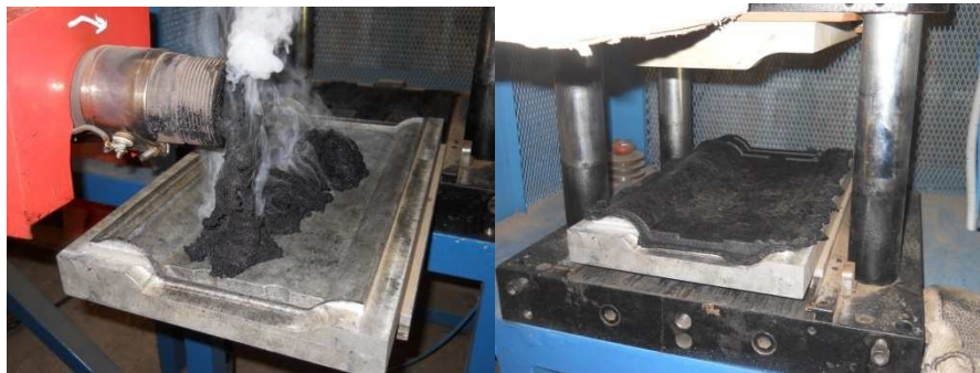
Figure 2 – Extrusion process and pressing of roof tiles.
