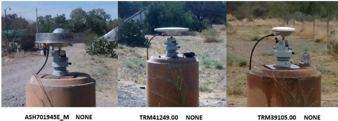
**Figura 2.** Antenas inclinación 0° (Ashtech Choke Ring, Trimble Zephyr Geodetic, Trimble Zephyr).
