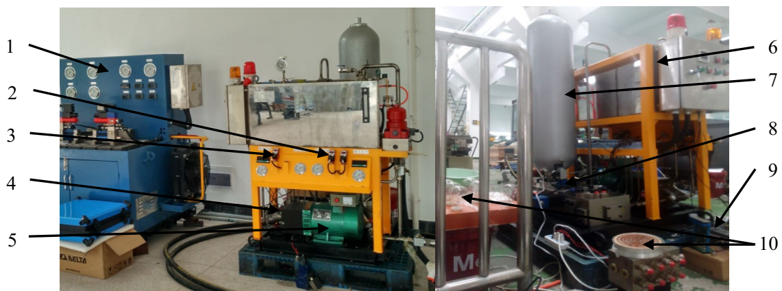
Fig. 7 IWEG wave energy capture, storage, and electrical power generation test rig. (1) Power pack, (2) hydraulic pressure sensors, (3) flow sensors, (4) hydraulic vane motor, (5) single-phase synchronous
