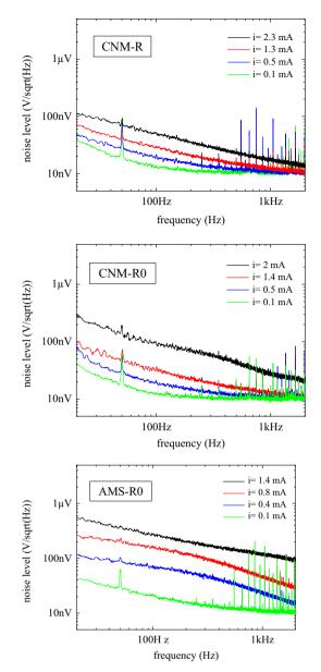
**Fig. 4.** Noise level (amplitude spectral density, ASD) at several bias currents for the different devices: CNM-R, spin valve onto current strip in a CNM chip; CNM-R0, spin valve onto free substrate in a CNM chip; AMS-R0, spin valve onto free substrate in an AMS chip.
