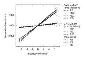
Fig. 3. Resistance of the deposited spin valve against the external magnetic field.
