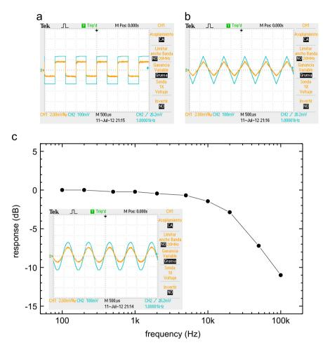
Fig. 7. AC behavior of the CNM 2.5 µm based devices as current sensors: (a) output for a square wave (1 kHz) driven current, (b) output for a triangular wave (1 kHz) driven current, and (c) frequency response to a sinusoidal driven current and output for such a wave at 1 kHz.
