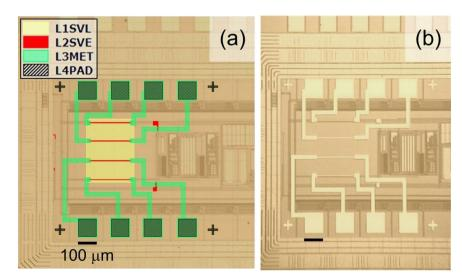
Fig. 1. Micrographs of the AMS chip with spin valves: (a) detailed masks, and (b) finalized process.
