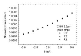
Fig. 5. Resistance of the deposited spin valve against the driven current in a CNM 2.5  $\mu m$  technology chip.
