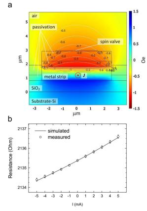
**Fig. 6.** 2D-FEM model of the CNM  $2.5 \,\mu$ m based devices as current sensors: (a) model description including magnetic field distribution, (b) resistance of the spin valve against the driven current: experimental data and simulation results.
