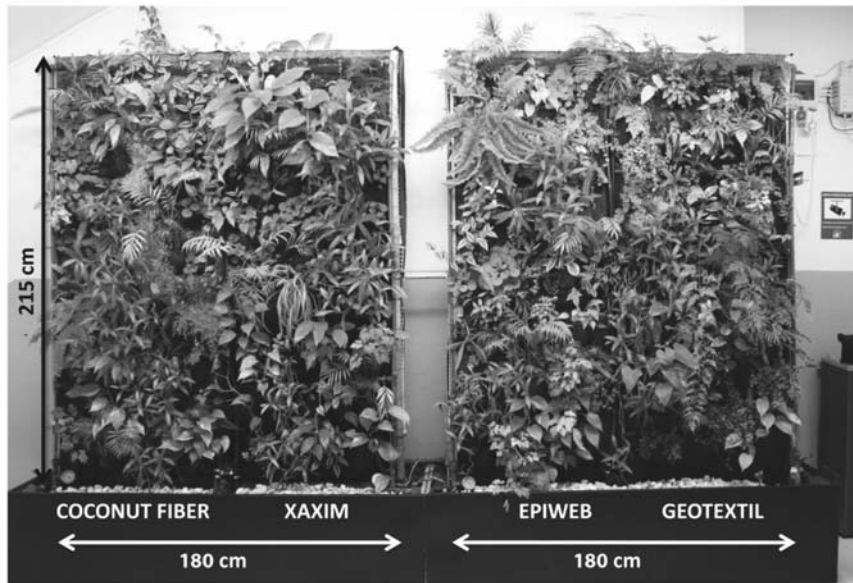
Fig. 1. Living wall and substrate disposition.
