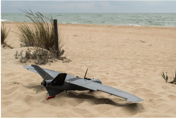
Figure 6.32 The Proskyttec-V1 is a 2000 mm wingspan fixed-wing V-tail UAV; manufactured with EPO, it has a maximum takeoff weight of 3.5 kg, also it has a fuselage length of 1220 mm, a surface area of 70 dm 2 . Its center of gravity is located at 100mm from the leading edge.
