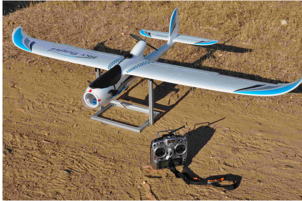
Figure 6.31 The SkySurfer X8 is a 2000 mm wingspan fixed-wing gliding UAS; manufactured with EPO, it has a maximum takeoff weight of 1.7 kg. The fuselage length is 1.35 m, it has a total surface area of approximately 46.3 dm 2 and a loading area of approximately 29.2 dm 2 , its center of gravity is located at 75 mm from the leading edge.
