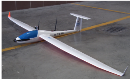
Figure 6.5 The glider utilized to perform the initial testing of the FDES wind-related functionalities.
