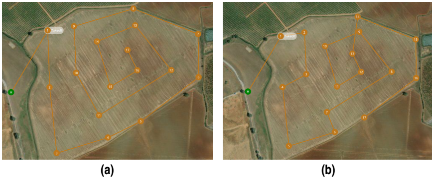
Figure 6.52 Two missions performed with the Proskytec V1 in the region of Brenes, Seville. The mission in (a) shows a surveillance mission with 17 waypoints that go in spiral from the outside to the inside, which prevents overlapping. In (b) the same waypoints are reconfigured in accordance to the detected wind direction, which was reported to be coming from the south east, which is the lower left corner of the pictures.
