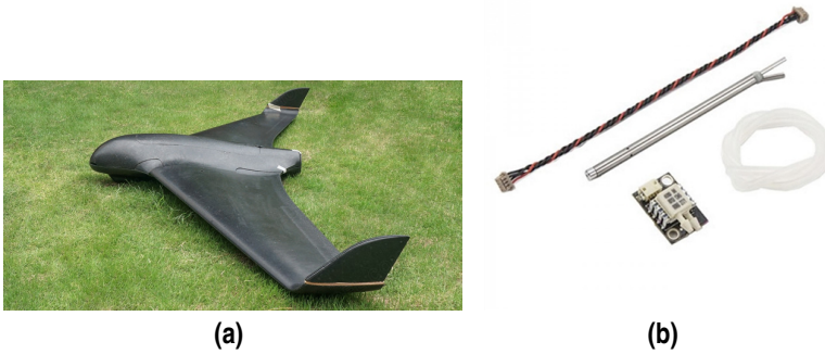
Figure 6.15 The SkyWalker X8 (a), from (SkyWalker Technology Co. Ltd, Wuhan, China) is a flying wing platform with a carbon fiber frame. The 4525DO sensor (TE Connectivity Ltd., Shaffhausen, Switzerland) with a resolution of 0.84 Pa [80].
