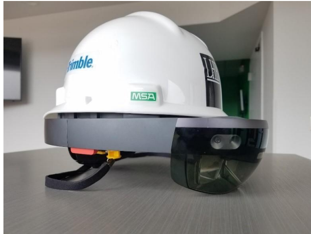
Figure 11 - Microsoft HoloLens integrated with a hard hat 11
