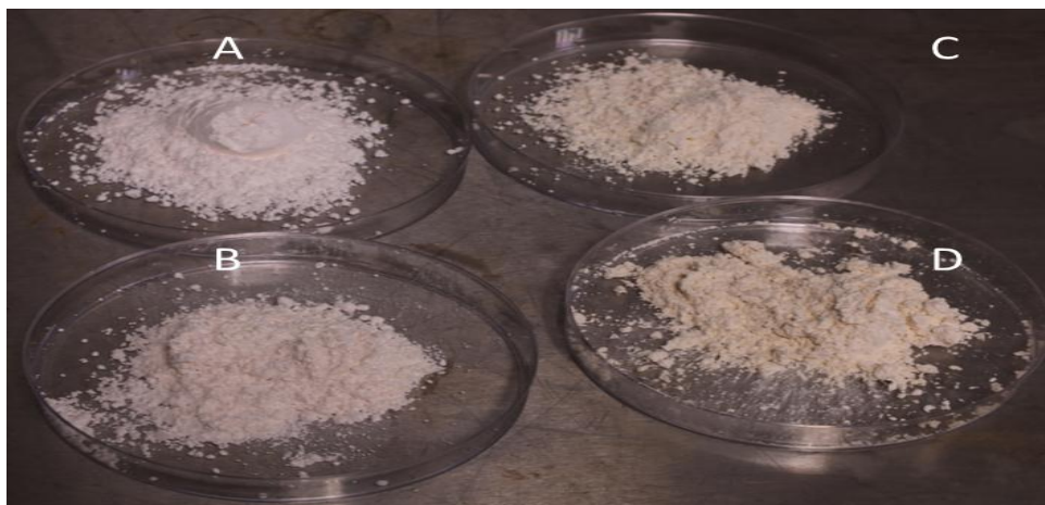
Figure VI–11. Powders obtained from spray drying. A-fruit 10% MD; B-fruit 15% MD; C-leaf 9+1%; D-leaf 10% MD.
