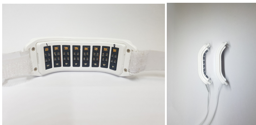
Figure 8. The optimized wrist surface type band by firmly attaching the PD array onto the wrist ( Left panel ). An examples of two bands with different curvatures optimized for: participants with small wrist (left in the right panel ) and participants with normal or thick wrists (right in the right panel ).
