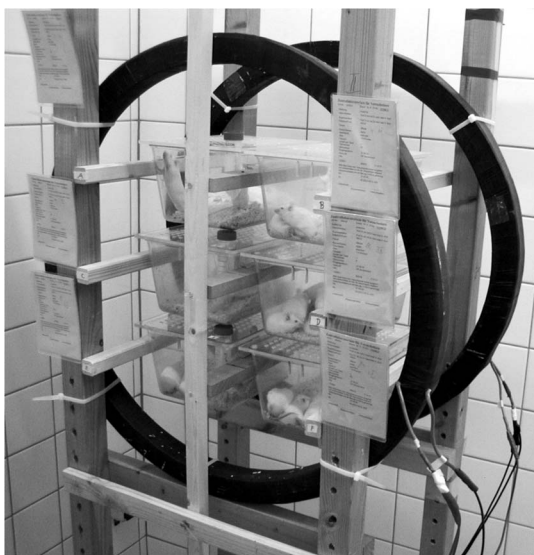
Figure 1. Experimental set-up of the 50 Hz MF exposure of the present study. Details are provided in the main text. doi:10.1371/journal.pone.0109774.g001
