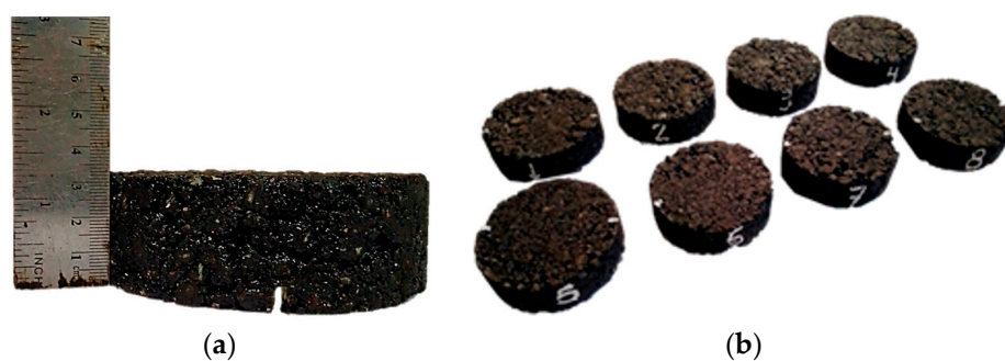
Figure 4. (a) Pre-notched sample; (b) Group of demoulded specimens.
