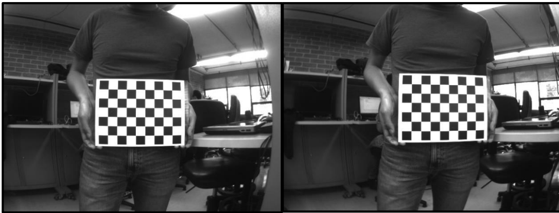
Figure 9. Example of stereoscopic images (left and right) taken for calibration
