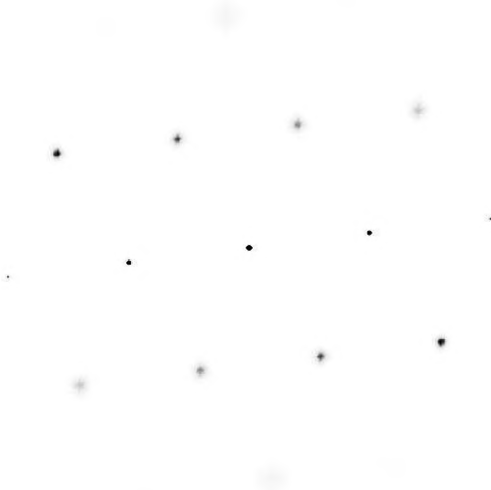
Figure S4: Stronger crumpling. A , Ripples are 0.5 nm in height and their typical size is 5 nm laterally. Ratio L/h is the same as in Fig. S3. B , Calculated diffraction patterns agree well with our experimental data.
