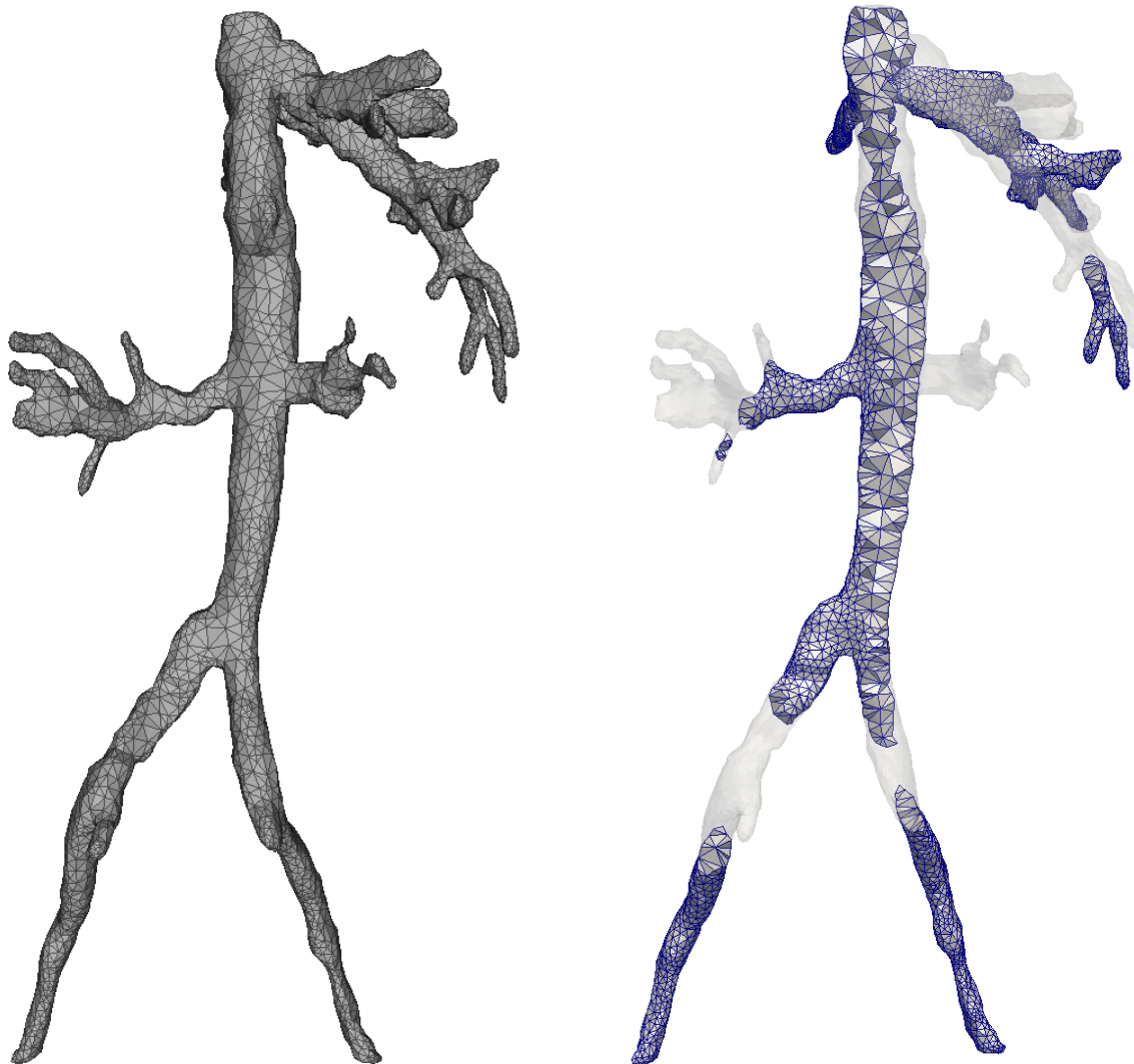
(a) BioCAD volume mesh of the venous system obtained from the implicit representation.
