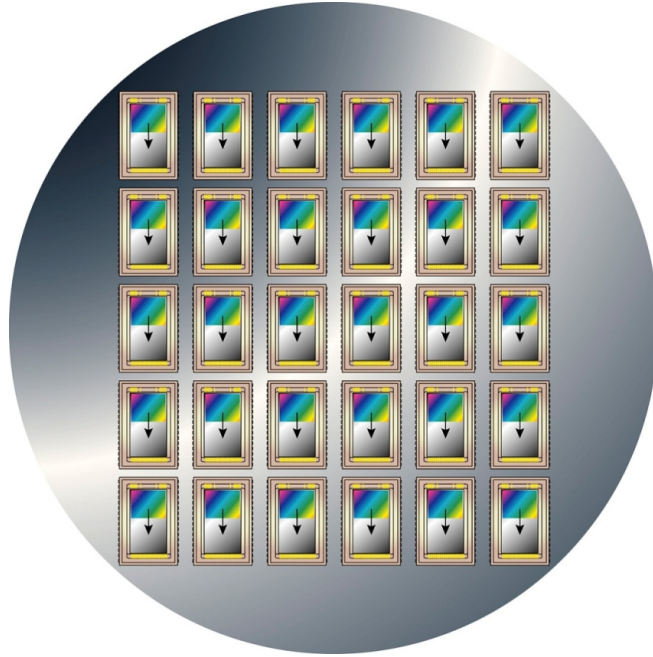
Figure 7. The detectors in GravityCam consist of a close packed array to fill completely the field of view of the telescope. The sensitive parts of the EMCCDs shown diagrammatically here only cover about 1/6 of the area of the detector package. Unfortunately it would be very difficult to re-engineer such devices to give substantially better coverage. Each detector has an image area plus a near-identical storage area. CMOS detectors have the attraction of offering at least 85% fill factor with current manufacturing technologies. CMOS imaging sensors are ubiquitous for many applications such as web cams and mobile phones, but not yet on large telescopes. However CMOS devices under development for astronomy are making rapid progress so are highly likely to be available for use in GravityCam.
