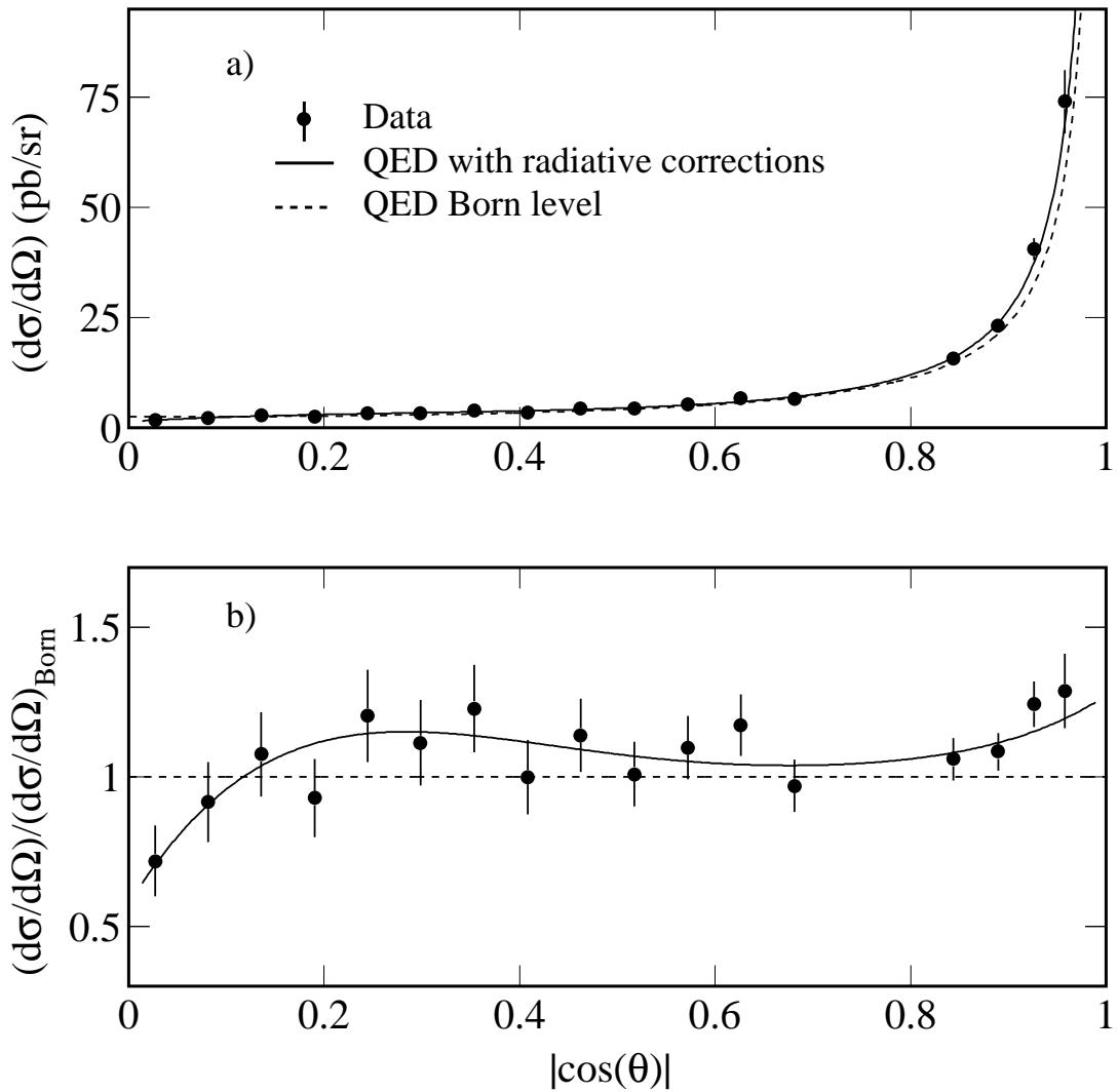
Figure 3: (a) shows the comparison of measured differential cross sections with the QED predictions for the process  $e^+e^- \rightarrow \gamma\gamma(\gamma)$  as a function of  $|\cos\theta|$ . (b) shows the same cross sections normalized to the QED Born level prediction.
