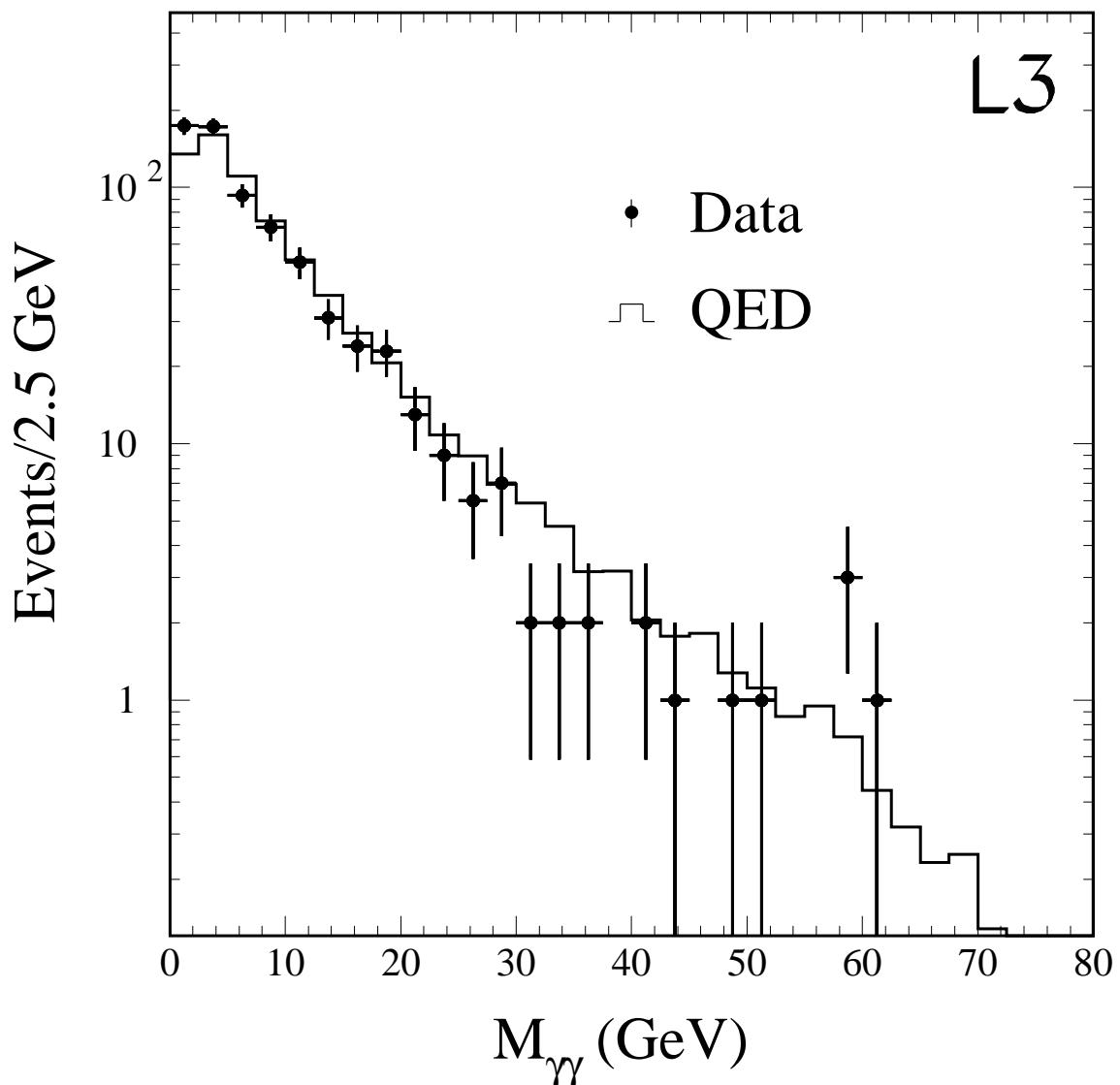
Figure 5:  $\gamma\gamma$  invariant mass distribution compared to the QED predictions for the process  $e^+e^- \rightarrow \ell^+\ell^-\gamma\gamma$ .
