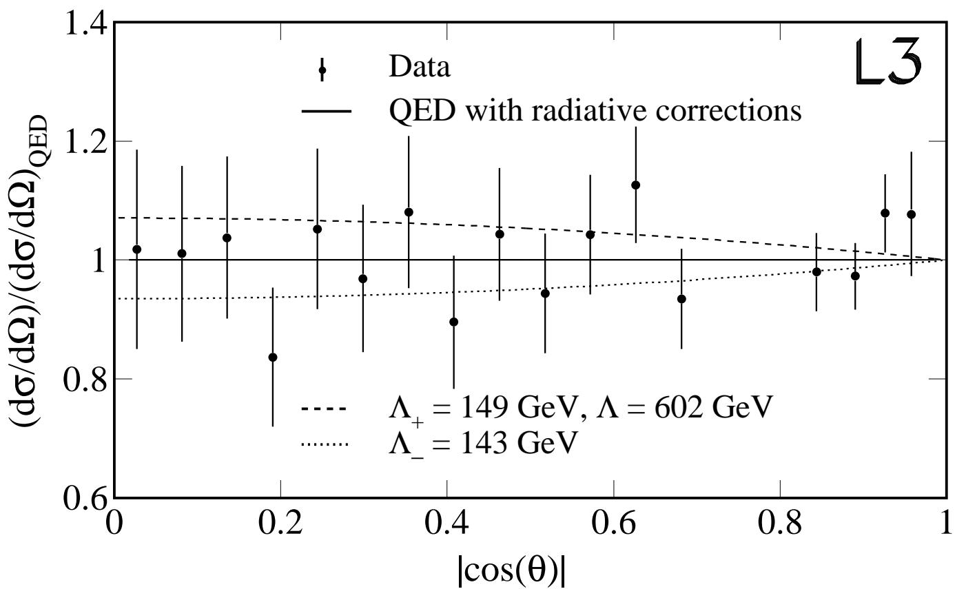
Figure 4: Comparison of the measured differential cross section with the QED predictions including the deviations for the parameter values shown in the figure, as a function of  $|\cos \theta|$ . The cross sections are normalized to the radiatively corrected QED cross section. The functional effect of  $\Lambda_+$  and  $\Lambda$  is the same.
