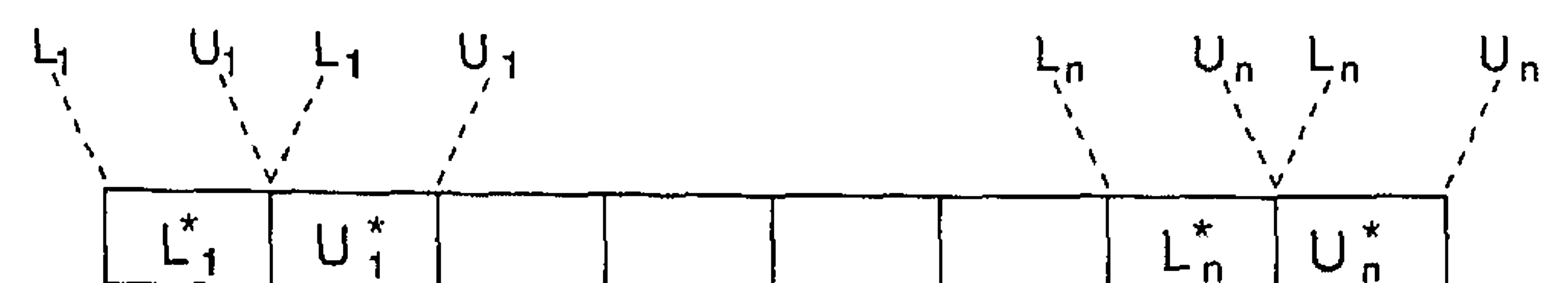
Fig. 2. Example of a trial solution (string). Each restraint is encoded on the string by using the real values of the lower and upper bounds. Each lower and upper bound is constrained by the corresponding original bounds.
