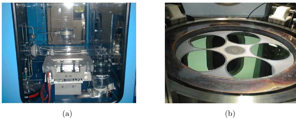
Figure 7: Aixtron reactors, (a) single 2 inch wafer R'n'D reactor and (b) multi-purpose industrial reactor capable of 5x10 inch or 95x2 inch wafer runs (5x10 inch Si wafers shown).
